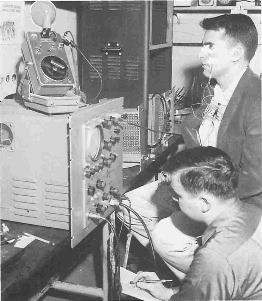
Figure 6-12. Medical research has many uses for the Strobotac. In above experiment, strobe helps researchers study eye behavior.
