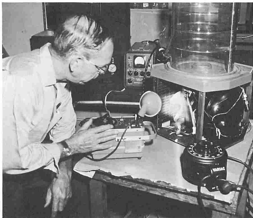
Figure 6-16. Technician uses Strobotac to troubleshoot cold-drink vending machine. Smoke can be added to trace flow of cooling air from the fan.
