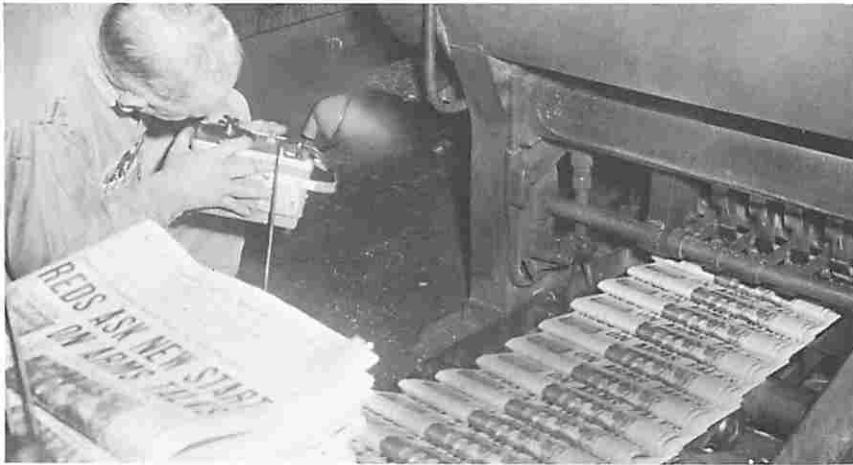
Figure 6-11. Strobotac is widely used to check press operation, color registration, etc. The faster the press operates, the more effective the Strobotac.
