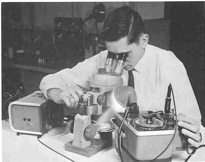
Figure 6-4. Engineer studies speaker cone under microscope while adjusting flash delay to divide oscillator output frequency down to stroboscope range.
