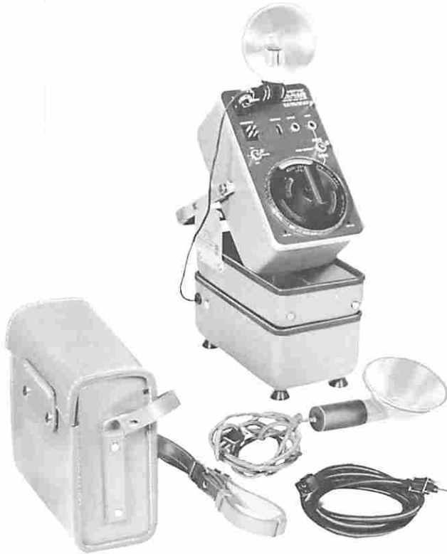
Figure 2-3. GR 1538-A Strobotac electronic stroboscope with accessories. Left foreground, in leather case, are battery and charger. Power cable is in right foreground, and extension lamp is next to Strobotac, which sits atop plug-in high-intensity-flash capacitor.
